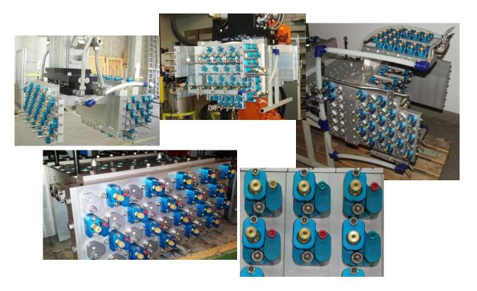
**Flextool™ from AED Automation** is a highly efficient spray technology for Pressure Die Casting to cool and lubricate dies. It has set industry standards for cooling and lubrication of PDC dies in shortest time. Its features are
